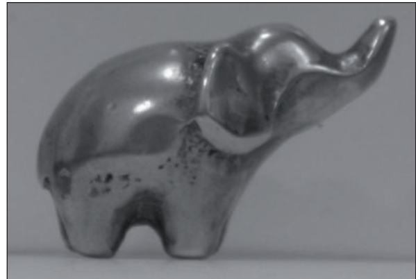
Figure 1. Surface porosity visible on a casting
