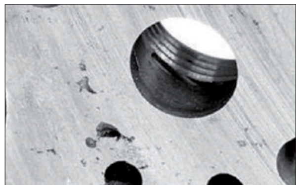
Figure 2. Internal porosity visible on a machined face
