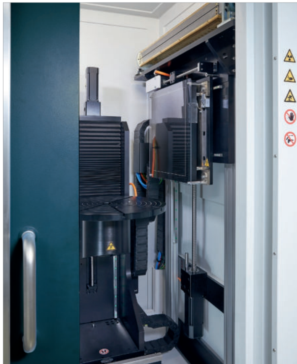
3D CT analyses of dense castings with line- or flat-panel detector of the UX50.
