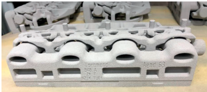
3D-printed, inorganic core for the cylinder head of the B48 engine.
