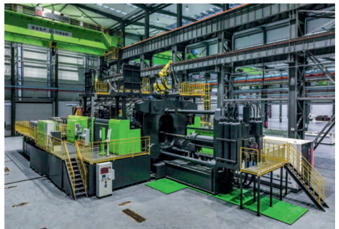
2022 LEAP die casting cell with 90000 kN of locking force for the production of ultra-large structural castings
