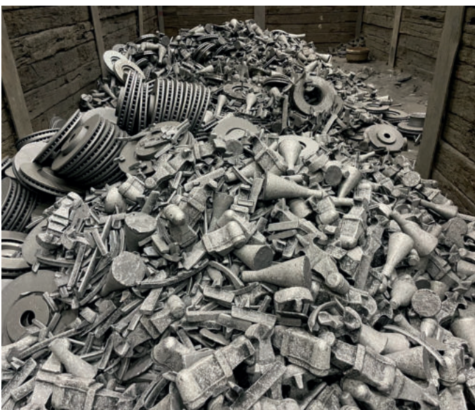
Cleaned and crushed returns ready for remelt in scrap yard.
