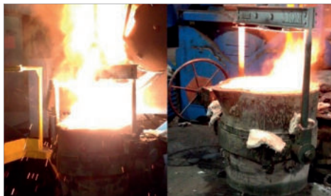
Reaction with steel coins covering MgFeSi (left) and using Topseed® Conditioner (right).
