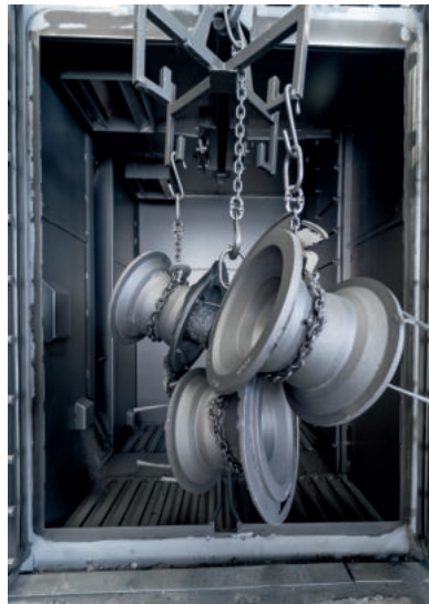
Workpieces after the blasting process in an AGTOS hanger type shot blast machine
