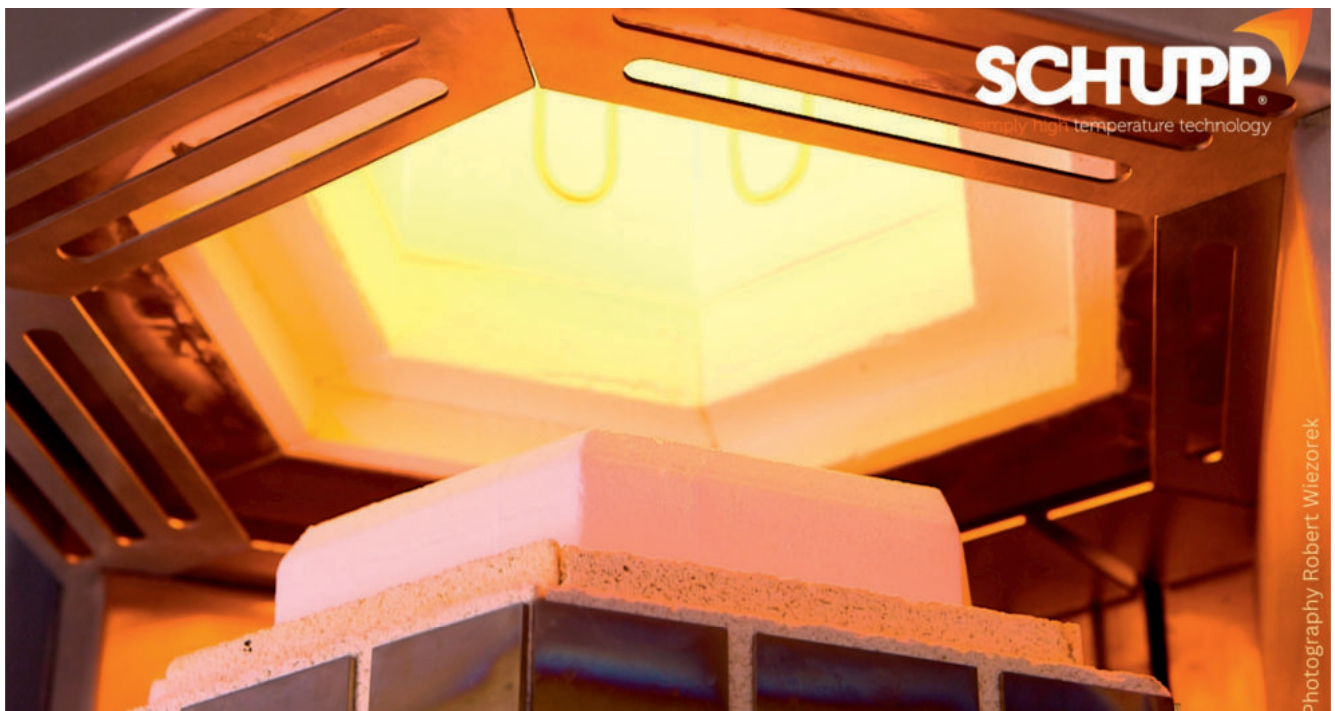
High-temperature furnace with electrical heating elements MoSi2.
