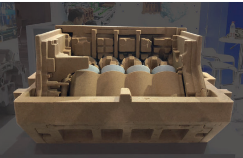
Engine Block Core using PCP Technology.
