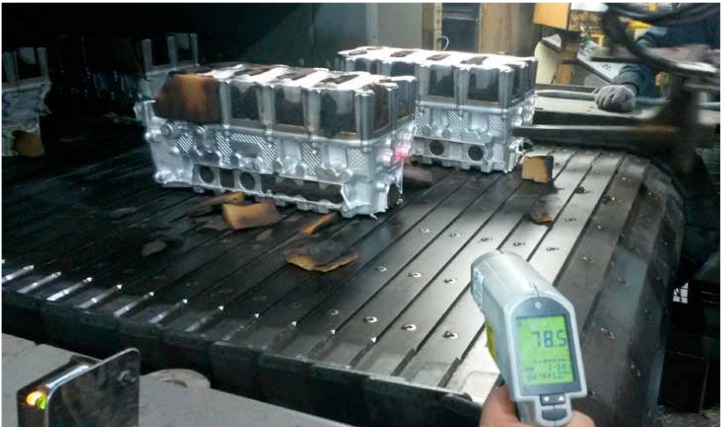
Aluminium engine heads outlet temperature with pyrometer.jpg
