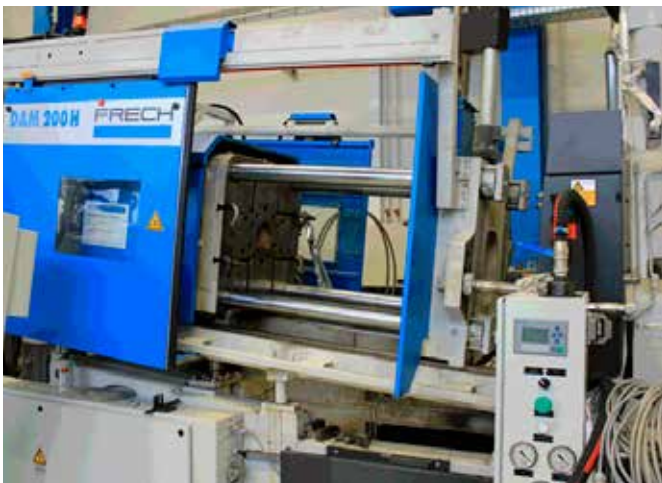
The hot chamber pressure die-casting machine used in the Frech technique for the production of salt cores (photo: Klaus Vollrath)
