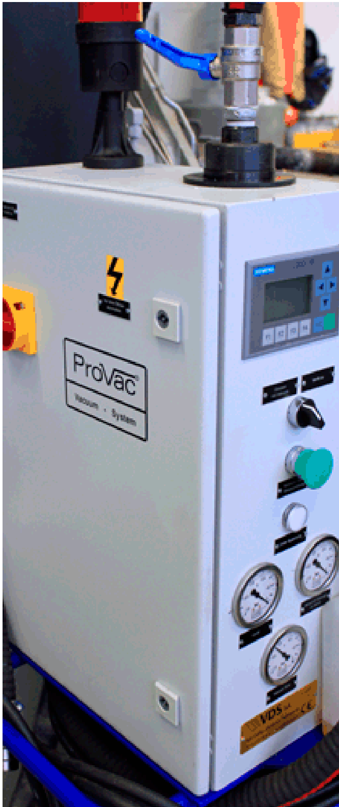
The system for mould venting detects the point in time at which the melt replenishment is interrupted and issues the signal for the subsequent pressure build-up for optimum compression (photo: Klaus Vollrath)
