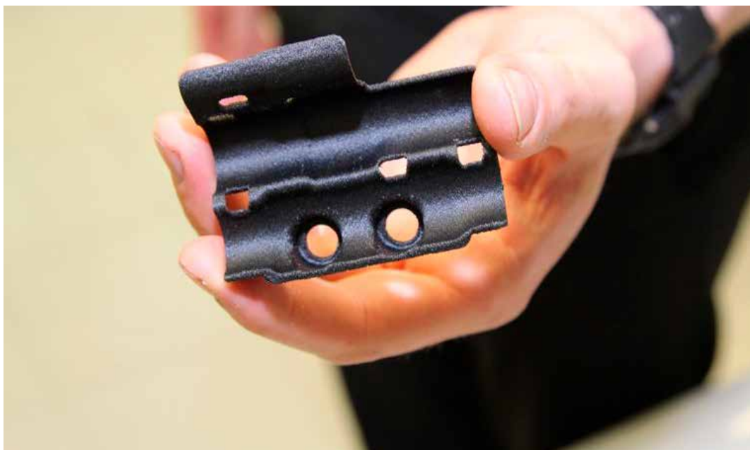
Hydraulic line bracket for the McLaren MCL32 race car, 3D printed on a Stratasys FDM 3D Printer using Nylon12CF material
