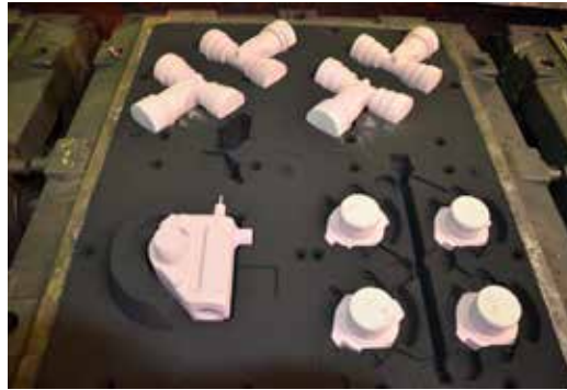
Düker produces most of its core product range with the new binder ECOCURE BLUE.
