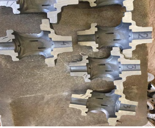
4 castings per box, all sound with good structure
