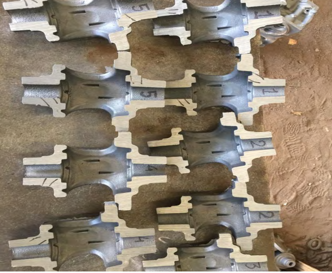
5 castings per box, all sound with good structure and properties
