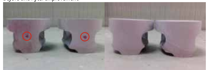
a) Shrinkage Cavity On the Casting Side Before Improvement
