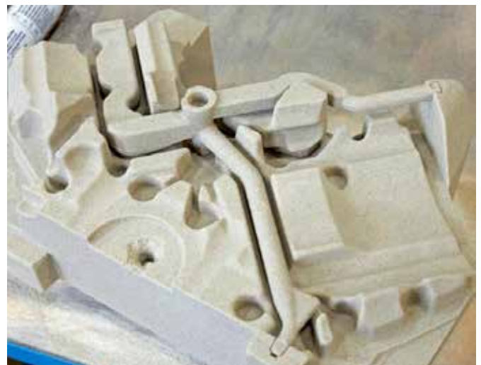
Example: Complex sand core with sophisticated three-dimensional varied geometry for a sand mould (photo: Klaus Vollrath)
