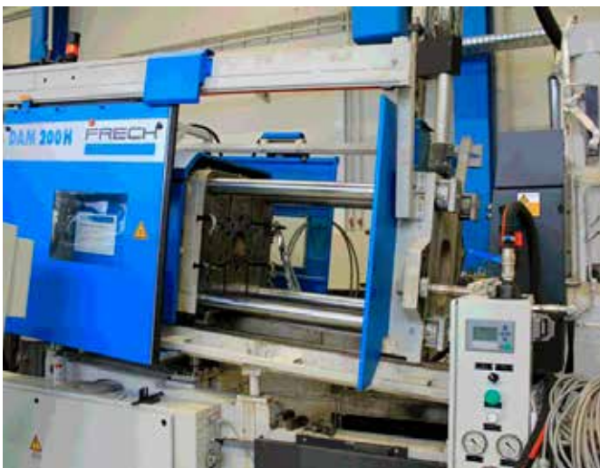
The hot chamber pressure die-casting machine used in the Frech technique for the production of salt cores (photo: Klaus Vollrath)
