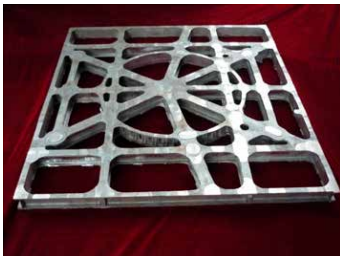
Bottom Structure Body of the Load Cabin of a Certain Model (2300 mm X2100 mm X110 mm, and 6mm Wall Thickness)
