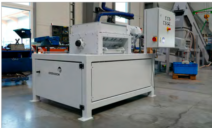
The M600/1 single-shaft shredder has been designed for die-cast parts weighing up to 2 kg and is available in two cutting gear sizes - 400 x 500 mm or 600 x 500 mm length and width - depending on requirements, as well as with a drive power of between 5.5 and 9.2 kW. (Source: Erdwich Zerkleinerungs-Systeme GmbH)
