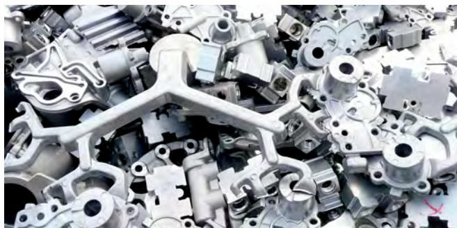
The handling of bulky sprue and runners, punch burrs and defective workpieces is a problem not only in zinc die casting, but also across the board in many light and non-ferrous metal foundries, which impairs the optimum process flow and thus the efficiency of production. (Source: Stihl024/stock.adobe.com)
