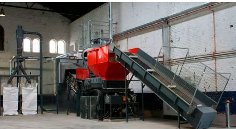
The H480/2 twin-shaft shredder is suitable for mid-size components up to 10 kg. Like the M465/2, it has a precise cutting gear with blade shapes adapted to the material and optimal feed behaviour due to the individual insertion options for the blades on the hexagonal shaft. (Source: Erdwich Zerkleinerungs-Systeme GmbH)
