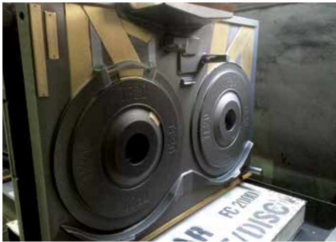
Picture 4: Pattern plate of a DISA 240-C
