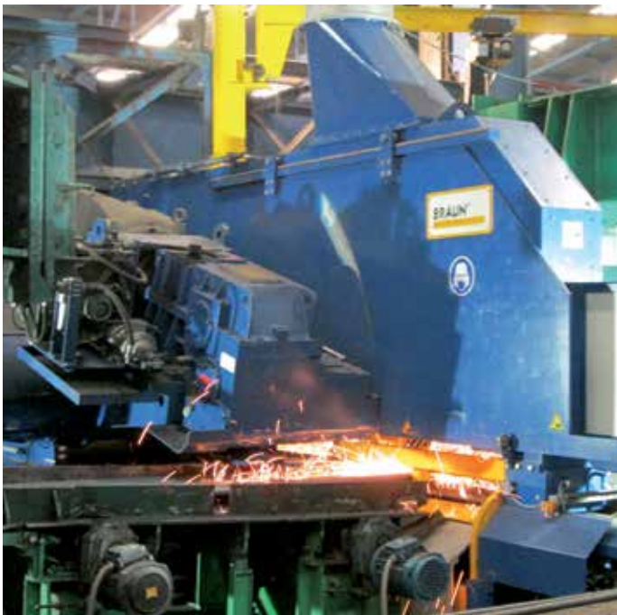
BRAUN cut-off machine type TS 12 F for upgrading NTS / TATA's existing bar mill in Chonburi.
